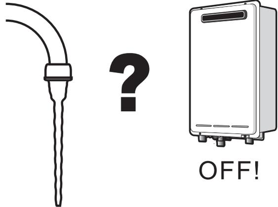
The delivered water temperature is controlled automatically. The water from the hot tap may be reduced after the temperature shown on the remote control is raised. The water flow may also vary with the temperature of the incoming water supply.
